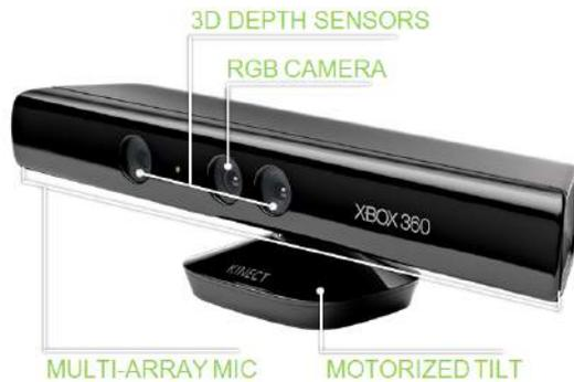
Figure 1. The Microsoft Kinect Sensor with its various streams identified
